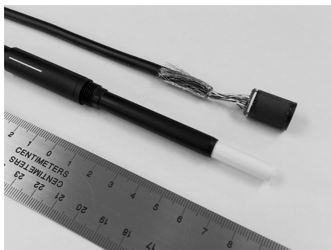
Fig. 12. A prototype of the Graphite Probe Calorimeter without its waterproof housing, next to a Sun Nuclear SNC 600c Farmer chamber for scale. The cylindrical graphite core (not visible) has a length of 10 mm and a diameter of 6.1 mm.
