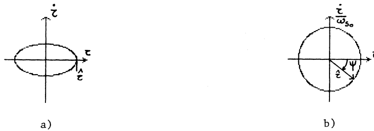
Fig. 1 Synchrotron motion in phase space. a) Phase space (\tau, \dot{\tau}) b) Normalised phase space (\tau, \dot{\tau}/\omega_{s_0}) or (\tau, \psi)
