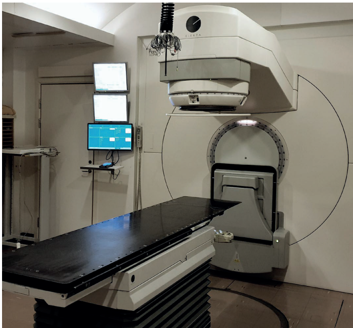
Figure 4: Photograph of the Elekta Precise linear accelerator modified for ultra-high dose rate delivery, which is used in the work throughout this thesis.
