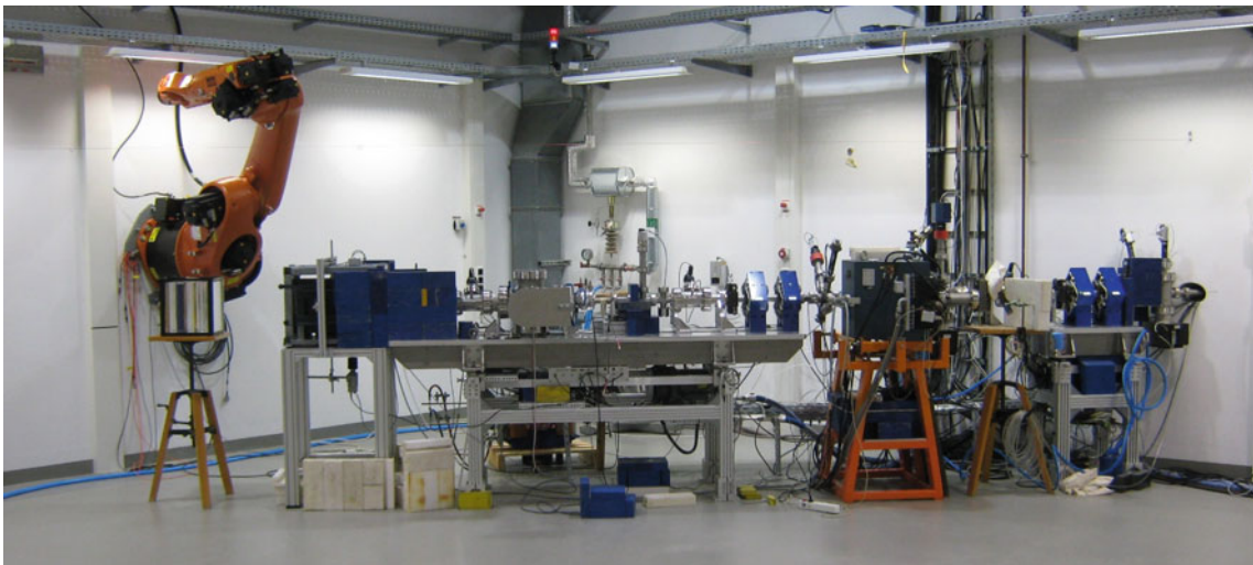
Fig. 2 Photo of the 6–50 MeV beam line of the research LINAC (beam enters from right)
