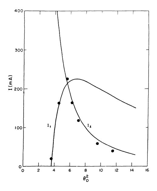
Fig. 1. Limiting beam currents vs  $\theta_0^2$  for an RFQ. The curves are obtained from the formulas 40 and 46 given in the text. The solid points are obtained from the computer program PARMTEQ.
